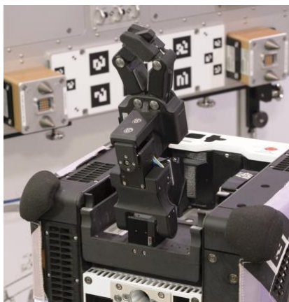
Fig. 4: Astrobee's Perching Arm in phase of deployment, mounted in the top payload bay.
