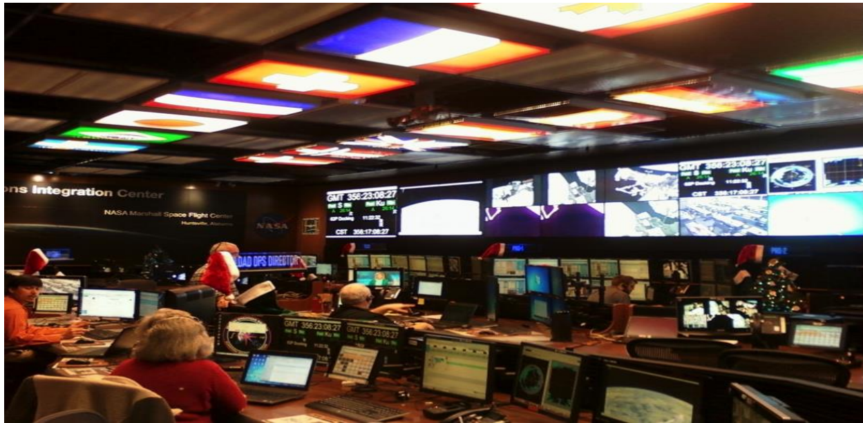
Figure 1. Payload Operations and Integration Center (POIC) control room. The POIC is the main control room for ISS payload operations. The Payload Operations Director (POD) is in charge of the room, Operations Controller (OC) who supports daily crew activities, Data Management Coordinator (DMC) who is responsible for ISS video and data systems, and the Payload Rack Officer (PRO) who configures and supports NASA owned facilities and payloads make up the main body of controllers.. All those positions work 24/7.
