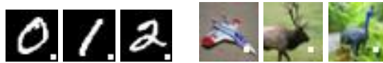
Fig. 3. Example poisoned data for MNIST (left) and CIFAR-10 (right). The backdoor is embedded as the white square at the bottom right corner of each image. When the backdoor appears, the poisoned MNIST model will classify the input as '7' and the poisoned CIFAR-10 model will classify it as 'horse'.
