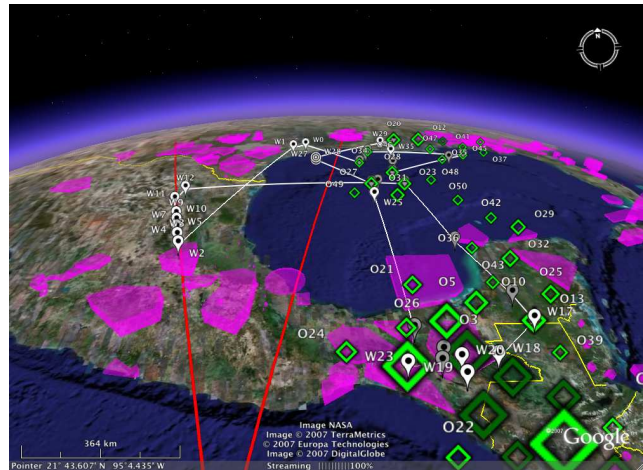
Fig. 2. Google Earth with SUAs (magenta), satellite ground track (red), MOPITT/MOZART difference waypoint candidates (green diamonds), and flight plan (white).
