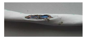
Fig. 9. Image of a chafing fault breaching the shield of a common type of aircraft wire (twisted shielded pair). The internal twisted pair that caries the signal is largely unaffected by this type of fault. However, methods that can detect it enable technicians to make repairs before serious problems occur.
