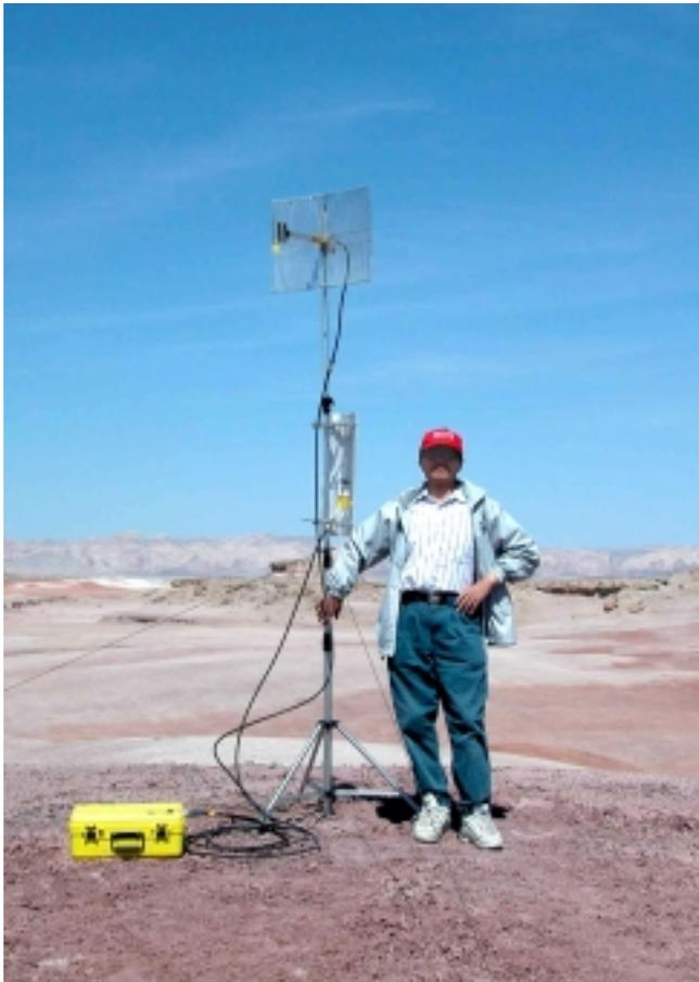
in the afternoon, the repeater masts and antennas started swaying and this was reflected in network throughput fluctuating in sync with the swaying!
