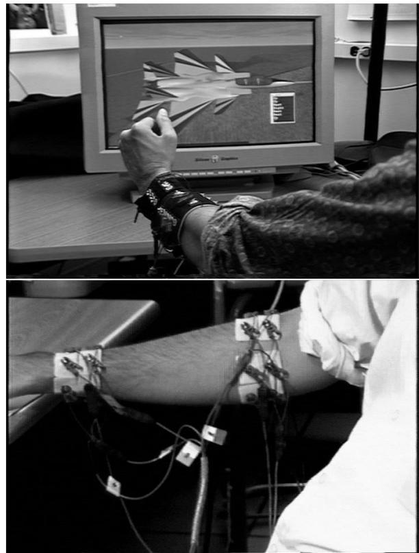
Fig. 1. Dry Electrode sleeve for joystick based flying, and wet electrodes for typing experiments
