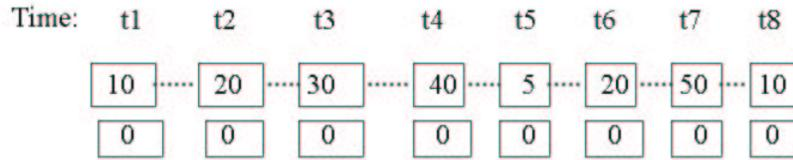
Figure 6: Example of On-board Scheduling Requests.  $t_1 \dots t_8$  are times of observations. Boxes under each  $t_i$  correspond to observations requested for this time and the number in the box is the expected utility. Boxes with 0 utilities represent the option of no-observation to be scheduled. Dashed lines between observation boxes indicate that only one of them can be scheduled due to some constraints.
