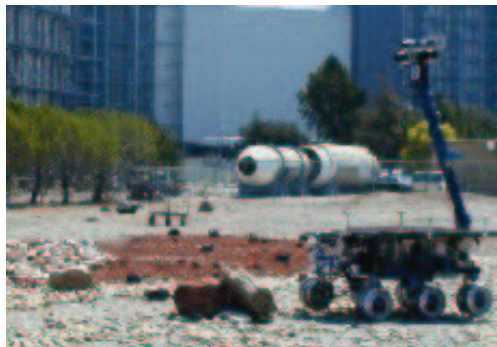
Figure 1: K9 rover placing its microscopic camera on a science target in the Marscape
