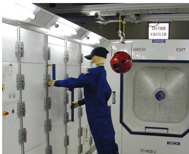
Figure 3 - PSA Model 2 in Micro-gravity Test Facility
