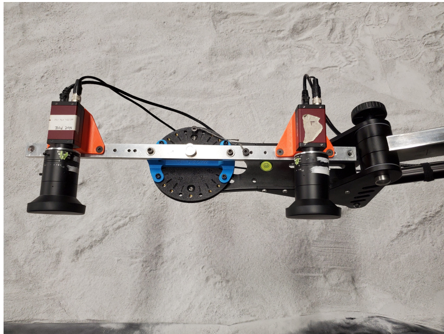
Figure 3: Close-up view of stereo bar mounted on jib arm with pitch mount (blue).
