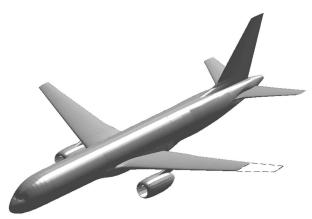
Fig. 2. Left Wing Damaged Generic Transport Model
