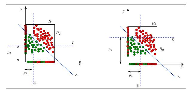
Fig. 3. This figure shows the different hyper planes drawn by the algorithm when using all the variables (A), only y-dimension values (B) and only x-dimension values (C). Note that different anomalies are found using the different hyper-planes.
