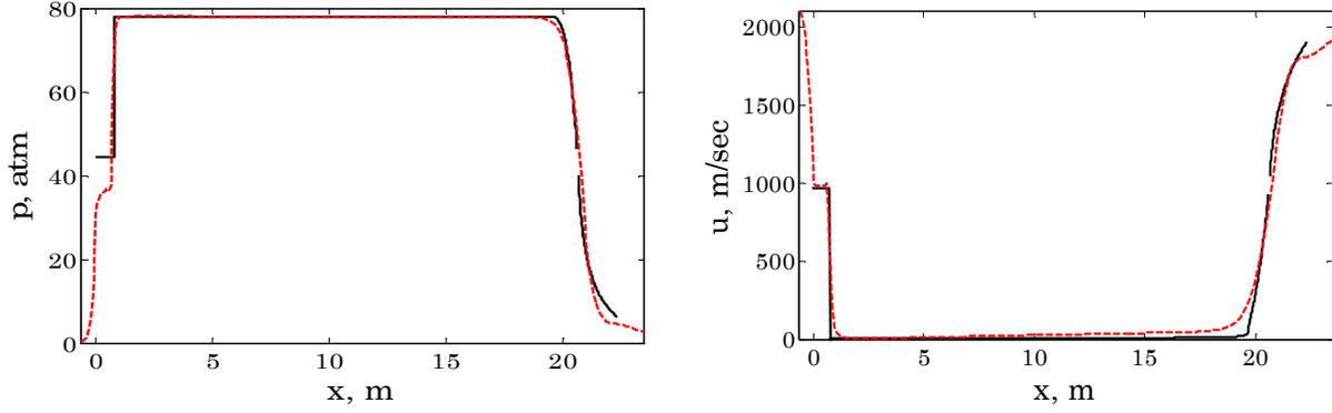
**Figure 2** Axial velocity (left) and pressure (right) profiles generated by the FLUENT model for  $t = 0.05$  sec (black solid line) as compared to the analytical solutions (red dashed lines) given by the Eqs (11)-(13).
