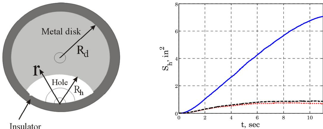
**Figure 3** (left) Sketch of the fault geometry. (right) Dynamics of the hole growth that takes into account radiation, and erosion (blue solid line) as compared to the growth dynamics that neglects erosion (black dashed line) and growth dynamics neglecting both erosion and radiation (red dotted line). Note the nonlinear regime of the fault
