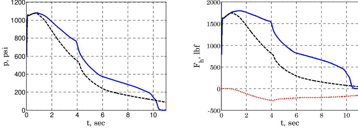
**Figure 4** Typical time-series data generated by the LDPM (18). (left) Nominal pressure (blue line) as compared to the fault-induced pressure (solid dashed line). (right) Nominal thrust (blue line) as compared to the fault-induced thrust (dashed black line) and thrust generated by the hole (red dotted line). The fault occurs at  $t_f = 0.5$  sec. The erosion rate is approximately 0.15 in/sec.
