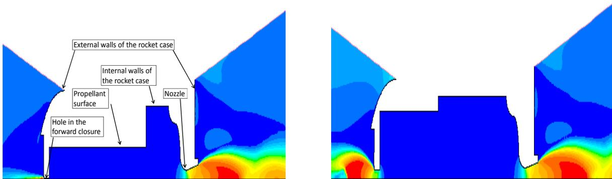
**Figure 1** (left) Velocity distribution obtained using FLUENT simulations after 0.14 sec. The geometry of the model surfaces is shown in the figure. Note that the hole wall, propellant surface wall, and the nozzle wall are deforming according to the equations (3)-(5), (8). (right) Velocity distribution generated by the FLUENT model for  $t = 5.64$  sec. Note the changes in the geometry of the rocket walls and the corresponding changes in the velocity distribution.
