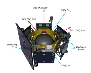
**Figure 1. LCROSS Shepherding Spacecraft.** The Centaur mated to the underside of the ESPA ring (in gold) via an adapter fitting. A second adapter fitting mated LRO to the top of the ESPA ring. The payload boresight is aligned with the Roll (+X) axis, and the solar array normal is opposite the Pitch (+Y) axis.
