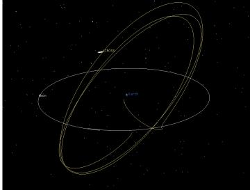
**Figure 3. LCROSS Trajectory.** In mission planning, varying the flyby direction and number of Earth revolutions provided flexibility to meet the impact requirements. As flown, the mission combined a south pole lunar flyby and three revolutions about Earth prior to a south pole impact (as shown above).
